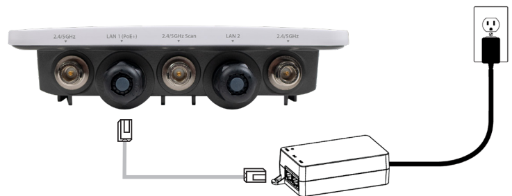
Access Point connected to PoE+ injector
